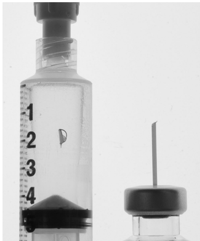
Fig. 2. Retained piece of the broken distal end of the blue dart in the syringe, with the other end in the vial.
